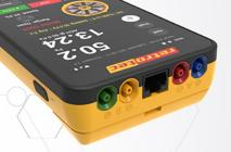
color coded pressure ports, cross compatible fan speed control, & magnetized belt clip
