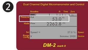
Fig 2: Fan adjusted to achieve about 50 Pa
