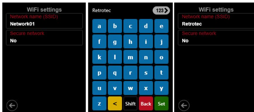
7. Press the “←” button to go back to the “Network settings” screen and wait for a number to appear as the “IP address”, which will appear once it is connected to the router. This should take a moment.
