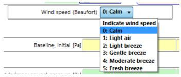
Choose the adjectives (from the Beaufort scale of wind speed) that best describe the wind speed during your test from the dropdown box.
