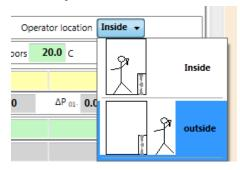
Select whether the operator is located inside or outside during the test (inside is typical). This is used in conjunction with the sign (positive or negative) from the Induced Pressure read from the gauge, to determine the test direction (Pressurization or Depressurization). The test direction will be displayed beside the Start time:
