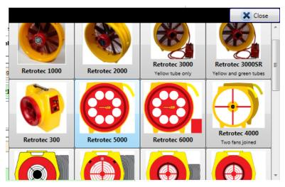
If you are performing a duct test, be sure to choose a Duct Testing fan, conveniently grouped together and shown in the picture with attached flex duct. Building test fans do not show the attached flex duct.
