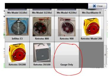
The pressure values on Channel A from the "Gauge Only" device are included in the room pressure. The pressure values read on Channel B and shown in the "No fan" line are not included in the flow calculations.
