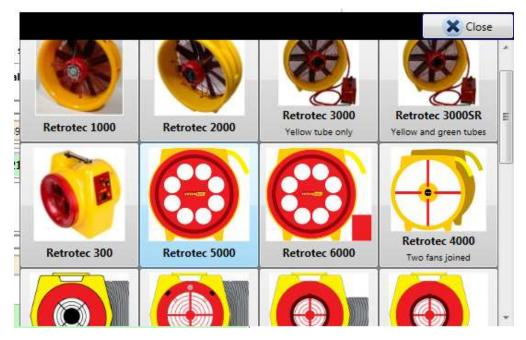
When you enter fan pressure values into the Test data set, you must have selected the device being used in order for FanTestic to correctly compute flow results. FanTestic uses the latest values of the Fan Flow Coefficients for each fan model to give you the most accurate value for flow.
