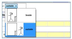
Select whether the operator is located inside or outside during the test (inside is typical). This is used in conjunction with the sign (positive or negative) from the Induced Pressure read from the gauge, to determine the test direction (Pressurization or Depressurization). The test direction will be displayed beside the Start time:
