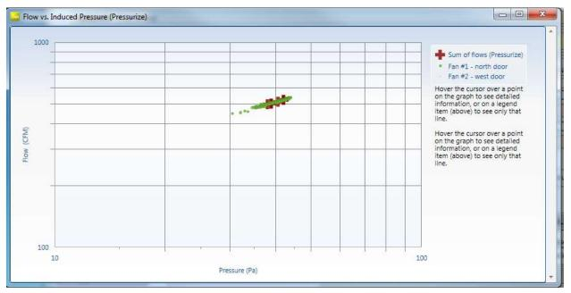
The number and location of the fan from which the readings are taken is shown on the graph legend, and moving the cursor over the points on the graph shows detail about each reading (pressure and flow at that point). The individual fan flow readings are shown, as is the sum of all flows in the case of the use of multiple fans.
