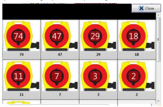
At the bottom of the Select Range chooser, you may also choose units for flow rates if you would like to manually enter flow rates by reading them directly off the gauge. If you only recorded flow values during a manual test, you will not have fan pressures to enter, so you must use this method.
