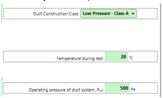
Based on the selected Duct Construction Class, the operating pressure of the duct system is set. This becomes the reference pressure for the test.
