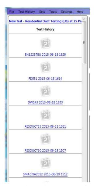
Make sure "New Test" on the history list is followed by the name of the Duct Testing Standard you are going to carry out. If not, go to "Settings" → "Change Standard used for new tests" and change the test standard. You may need to restart the program if this change is not active immediately.
