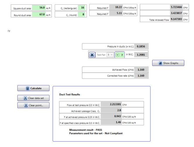
SMACNA provides a Leakage Factor  $C_L$  for each shape of duct which is used to calculate the maximum flow per area, F. The F for each shape of duct are then used to calculate the allowed flow for each shape, and the Total Allowed Flow is shown.
