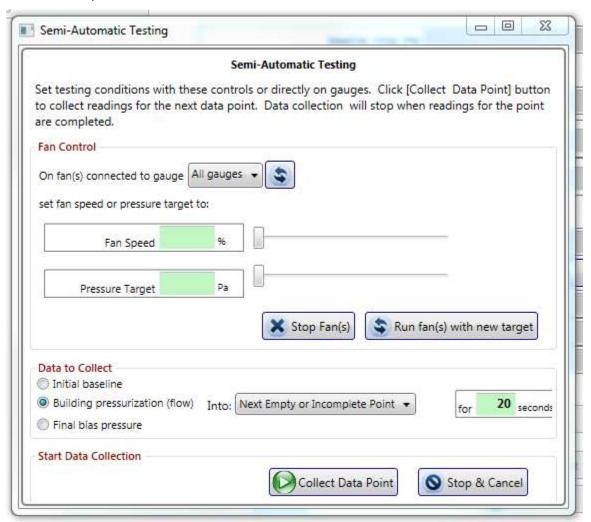
Fans can be controlled to reach a target pressure either by setting the speed, or by setting the target building pressure. Enter the target fan speed or building pressure into the appropriate green box, or use
