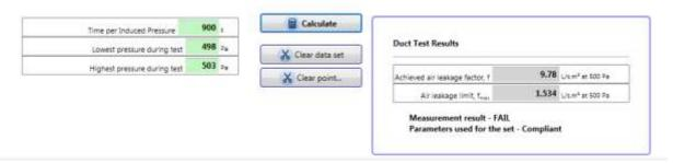
The Duct Test Results show the flow per square metre, f, that was achieved at the required test pressure (n = 0.65 for ducts). That f is compared to the maximum allowed flow per square metre to determine a measurement result PASS.
