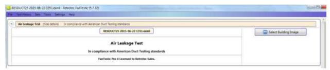
FanTestic is software designed to capture data and calculate results required for the analysis of building or duct air leakage based on one of a number of published Test Standards.
