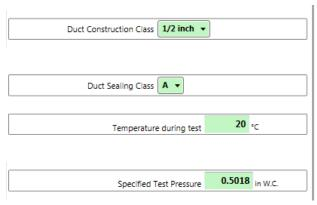
Based on the selected Duct Construction Class, the Specified Test Pressure is set. This can be changed by the user, but whatever this number is becomes the reference pressure for the test.
