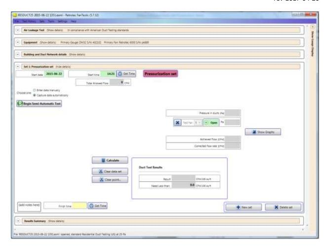
Data readings from each fan are specific to the range configuration installed on the fan when the pressure is read from the gauge. A Fan Pressure Line must be included in the set for each fan/range combination used during the test. New fan pressure lines must be added if ranges have to be changed during a test to reach the required induced pressure.
