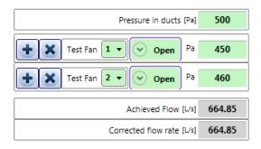
The results show the Achieved Flow and Corrected Flow at whatever pressure the test is carried out at. A visual check can be made, comparing the Total Allowed Flow with the resulting Corrected Flow to see if the test has passed.
