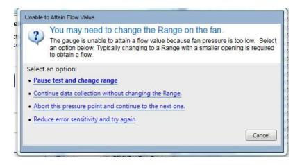
If you determine that you need to change the Range to complete the target point, click on "Pause test and change range", then physically change the range on the fan, and change the Range showing on the gauge. You will see the following in the Test Dashboard.
